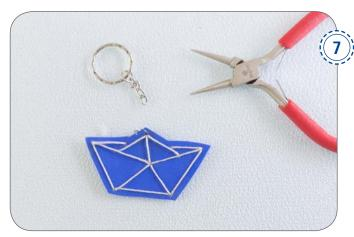
Use jewellery pliers to bend open a split ring, and feed it in through one of the top holes. Connect it to the key ring and bend it shut again.
